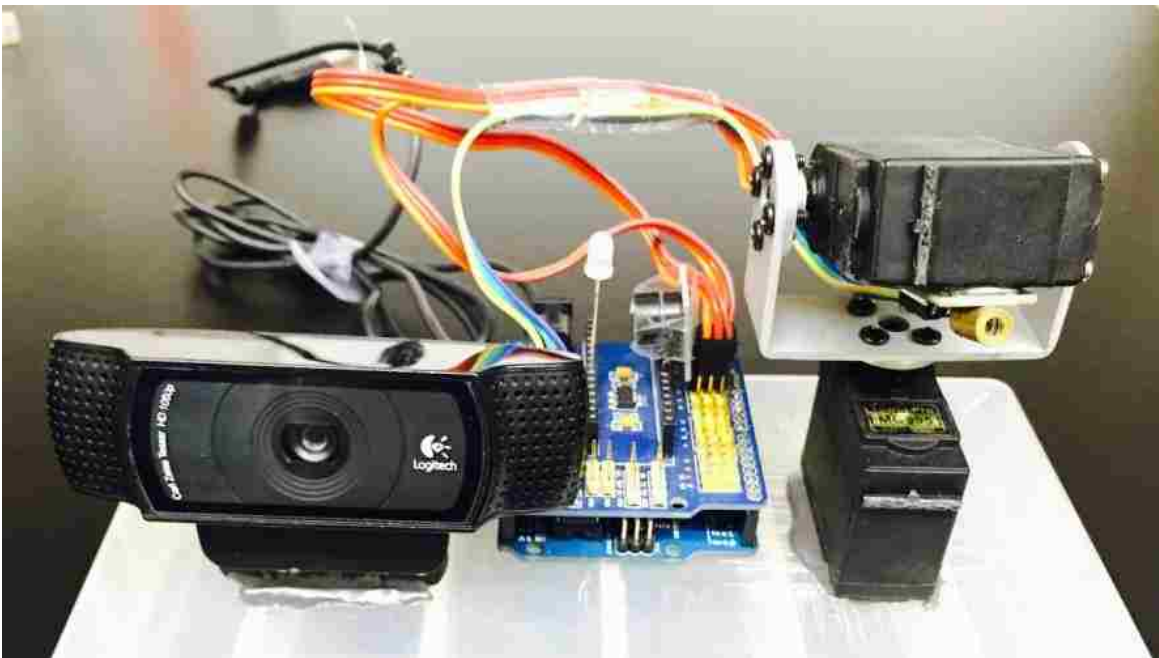
Figure 5: Prototype for drone detection and Tracking
